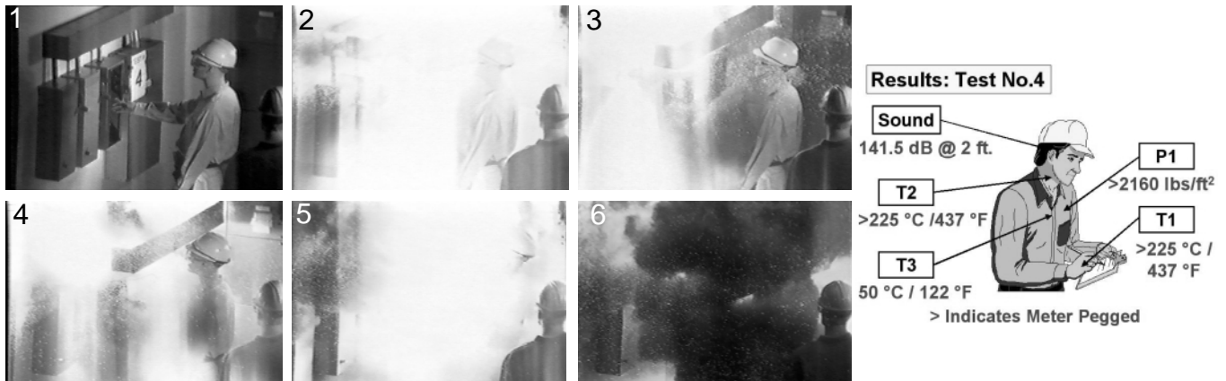
Photos and results Test 4: Staged test protected by circuit breaker with short-time delay (not a current-limiting overcurrent protective device). Short-time delay intentionally delayed opening for six cycles (0.1 second). Note: Unexpectedly, there was an additional fault in the wireway and the blast caused the cover to hit the mannequin in the head.
