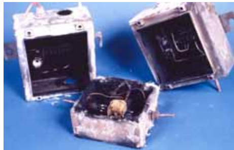
SX and BPG Range Enclosures after BS6387 Testing
