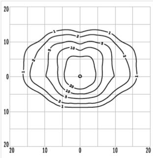
Flat glass with reflector in position 1 with 70 Watt SON-T lamp mounted at 5 metres
