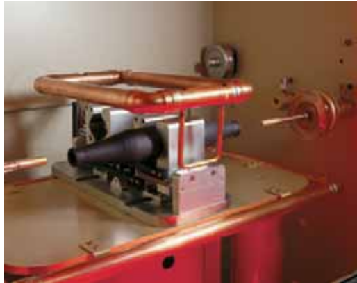
The premoulded cable joints are routine tested after manufacturing.
