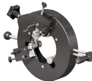
SH 50, SH 80, SH 130 Tool for removing and peeling XLPE-insulation and for removing outer conductive layer.
