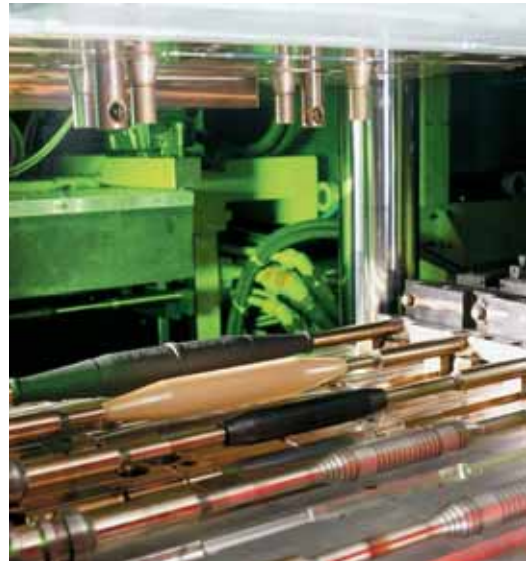
The three layers of the joint are vulcanized together in a unique manufacturing process.
