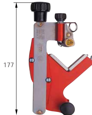
Intercable No. FBS 1722 1 Stripping tool for the vulcanized, outer conducting layer of XLPE-insulated cable Ø 10-52 mm. The tool is supplied in a rigid case with a tube of silicone grease.
