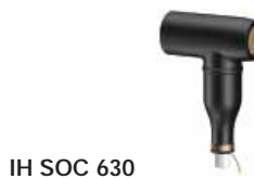
IH SOC 630 Insulating sealing hood of flexible rubber with outer conductive layer and an already installed insulating hood. To be installed in SOC instead of cable in order to temporarily insulating 630 A switchgear or transformer bushings.
