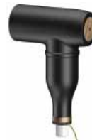
IH SOC 630 Insulating hood of flexible rubber with outer conductive layer and a preinstalled insulating rod. To be mounted on the bushing in a 630 A switchgear or transformer to insulate it when a cable is temporarily disconnected but other cables are energized.
