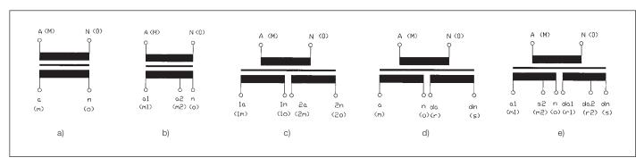
a) Single-pole insulated transformer b) Double-pole insulated transformer with a tap secondary windings, with one of which being the auxiliary (residual) winding binding.
