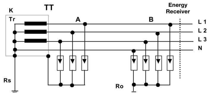
TT neutral point of transformer is earthed directly, while the receiver's installation is earthed by a separate earth electrode
