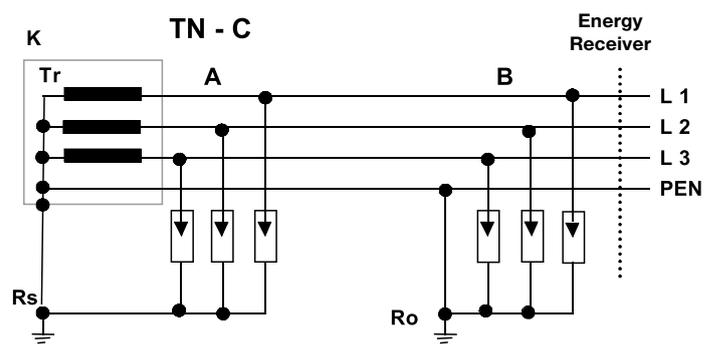
TN-C neutral and earthing conductor are common (PEN) and earthed at the transformer or near it
