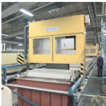
Automatic pre-treatment of enclosures before powder coating.
