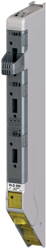
SLD 000 Fuse-switch disconnecter. - AC-23B according to IEC 60947-3 - 3 modules or 38 mm width - Fuse NH 000 or C00 - Sealing possibility
