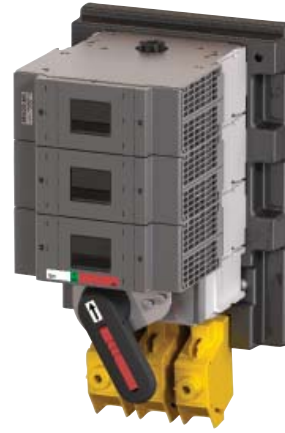
SEKOD 400 Switch-fuse with breaking on both sides of the fuse. Here SEKOD 400 in OFF position.
