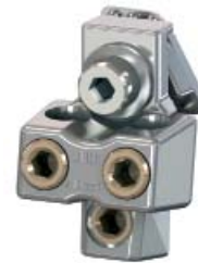
AD 350 Non-insulated connector for connecting three separate conductors, each max 50 mm 2 Al/Cu. May only be used with non-protected busbars.
