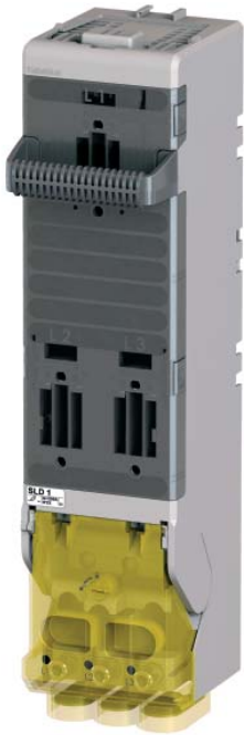
SLD 1 Fuse-switch disconnecter. – AC-23B according to IEC 60947-3 – 10 modules or 120 mm width – Fuse NH 1 (max width 42 mm)
