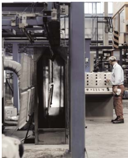
Powder coating of foundation parts.
