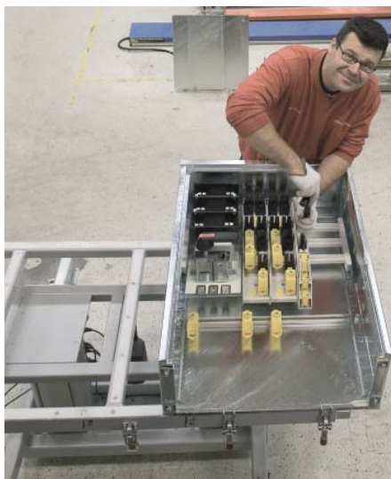
Assembly of distribution boards.
