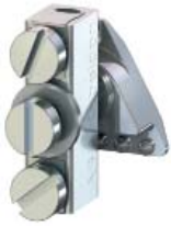
ADC 25 Non-insulated connector. May only be used with non-protected busbars for 1.5-25 mm 2 conductor.
