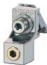
AD 70 Non-insulated connector. May only be used with non-protected busbars for 6-95 mm 2 cable.
