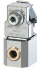
ADO 240 Non-insulated connector. May only be used with non-protected busbars for 120-240 mm 2 conductor.
