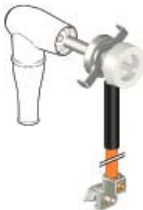
JP 250-HDC Earth circuit connector for short-circuit protective earthing. For mounting on the disconnected connector. 3 pieces in a case.
