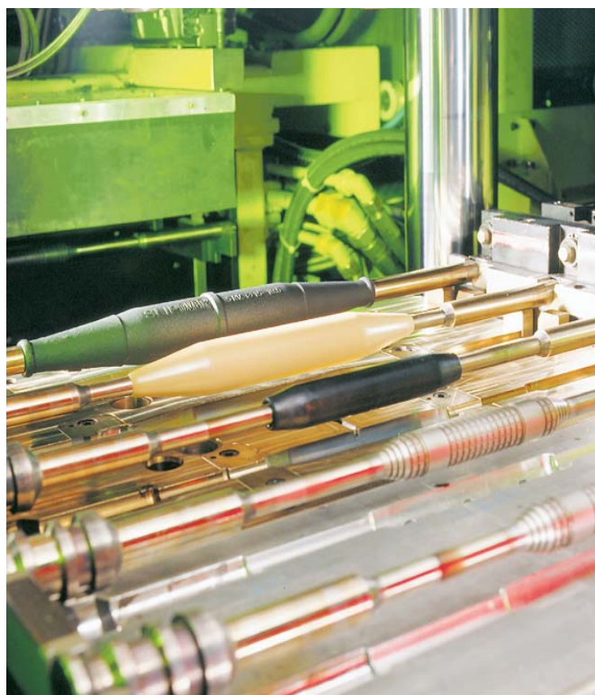
The three layers of the joint are vulcanized together in a unique manufacturing process.
