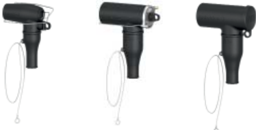
IH-A 24250, IH-A 24400, IH-A 24630 Insulating hood of flexible rubber with outer conductive layer and a preinstalled insulating rod. To be mounted on the bushing in a 250 A switchgear or a transformer to insulate it when a cable is temporarily disconnected but other cables are energized.
