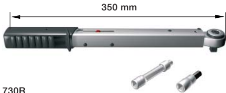
730R Torque wrench for bolt connectors, bolt cable lugs, overhead line clamps, etc. Supplied with 7 mm socket head, extension arm and 8 mm internal hexagon head. Torque range 6-50 Nm.
