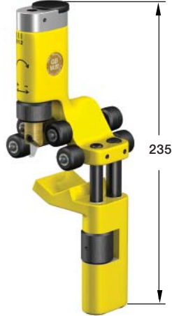
GB-M20 Cutting tool for cable sheath and XLPE-insulation: Diameter: Ø 15-50 mm Cutting depth: ≤ 8 mm
