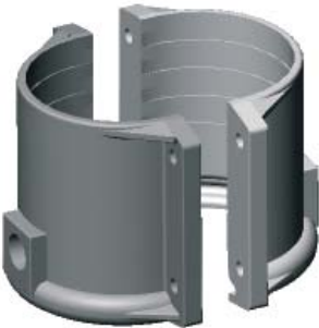
GC The kit contains one sealing ring, bolts and two roomy clamp halves for Ø 100 mm joint tubes. The clamps are made from glass fibre reinforced polymer. The bolt and washer are molded into the material. Used on the XLPE side of the transition joints; SMTXB 1502/1522/1532 when installing 1-core cables with an outer diameter greater than 40 mm.
