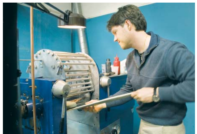
Manufacturing outdoor cable terminations for paper-insulated cables in 1962.
