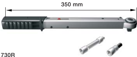
730R Torque wrench for bolt connectors, bolt cable lugs, overhead line clamps, etc. Supplied with 7 mm socket head, extension arm and 8 mm internal hexagon head. Torque range 6-50 Nm.
