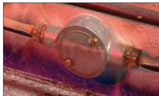
Appropriately jointed Firetuf cables continue to provide circuit integrity up to the full BS 5839 rating.
