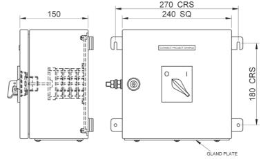
External Fixings - M6 Termination - M6 Stud Maximum Cable Size - 25 mm<sup>2</sup> Approx. Wt - 4.5 kg
