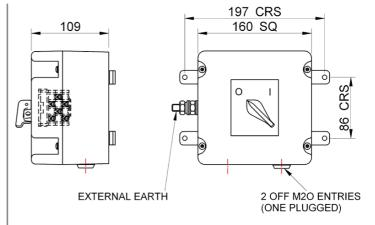
Termination - M4 Maximum Cable Size - 6 mm<sup>2</sup> External Fixings - M6 Weight - Approx. 2.5kg
