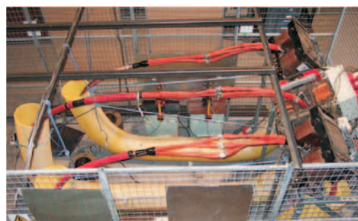
Picture shows XLPE and PILC 12kV Joints and Terminations undergoing type testing to BS 7888 and Cenelec standard HD 628 S1 and HD 629.1 S1 ASTA Test Report Available
