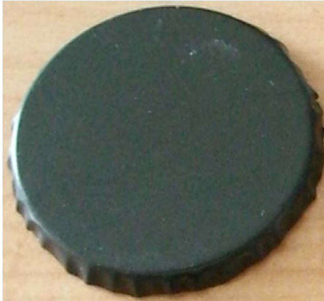
Picture 5: A test specimen after 16 weeks in salt water solution
