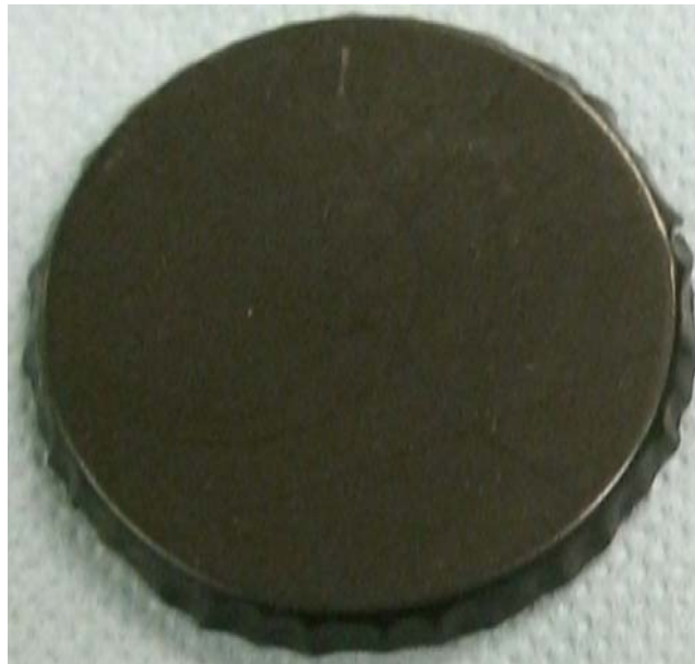
Picture 4: A test specimen after eight weeks in salt water solution
