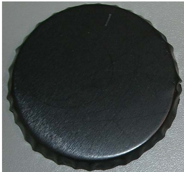
Picture 2: A test specimen after two weeks in 10% salt water solution
