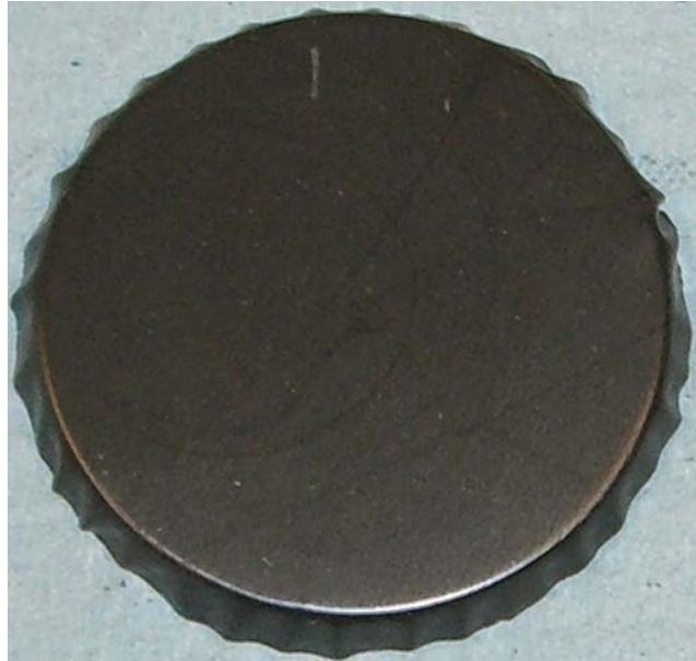
Picture 3: A test specimen after four weeks in salt water solution
