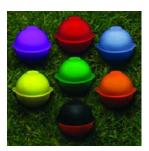
The 1402-XR 4" Extended Range Ball Marker has a self-leveling design insuring accurate, horizontal position regardless of how it is placed in the ground and making the job of precisely locating underground power facilities easier. The ball marker contains a passive-tuned antenna, molded inside a plactic disk, which is free-floating inside a waterproof, polyethylene shell. The ball marker has a range of five feet (1.5 m).
