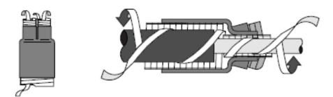
2. After measuring required length, install RJS – Series silicone rubber phase re-jacketing sleeves.
