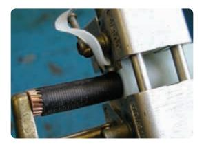
• The connector comes with metal inserts to fit small conductors. If the conductor will not fit the connector, discard the insert and use the connector without it.
