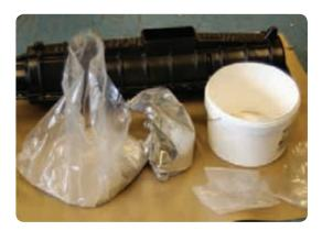
• Pick up the foil bag containing the resin and hardener and apply pressure to the large resin pouch so that the resin breaks the seal between the two sections and mixes with the hardener.
