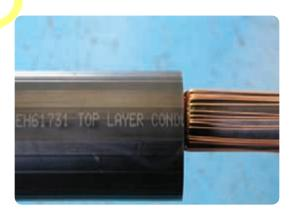
• Shrink the black and red tube down starting in the centre. When this section is fully shrunk it should be smooth without ridges and should not move when twisting the tube end.
