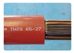
• Shrink the tubing down starting at the over-sheath end and working towards the insulating rod end.
