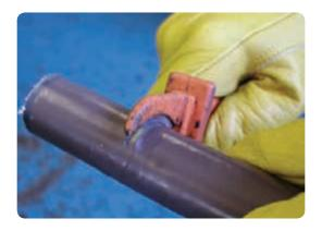
• Remove the clear barrier tube by pulling towards the end with a gentle twisting movement.
