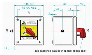
Internal Fixings - M6 on 85 x 85crs Termination - M4 Maximum Cable Size - 2.5 to 6.0 mm<sup>2</sup> Weight - Approx. 1.4 kg
