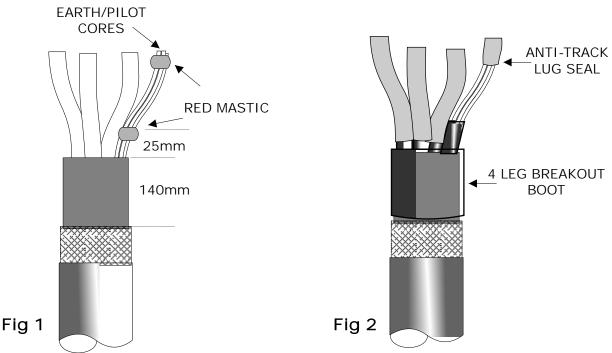
STAGE 1 Strip the Cable Bedding to approx 140mm. It is not necessary to applied Red Tape to the Bedding as the Breakout Boot is adhesive lined.
