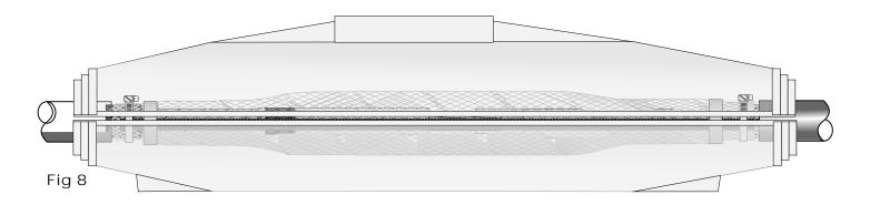
13. Clean/de-grease and abrade the outer cable sheaths. Position the joint shell so that it fits correctly to the cable diameter, trim the ends as necessary. Mix the resin according to the manufacturers instructions and completely fill the shell, replacing the filler cap supplied.
