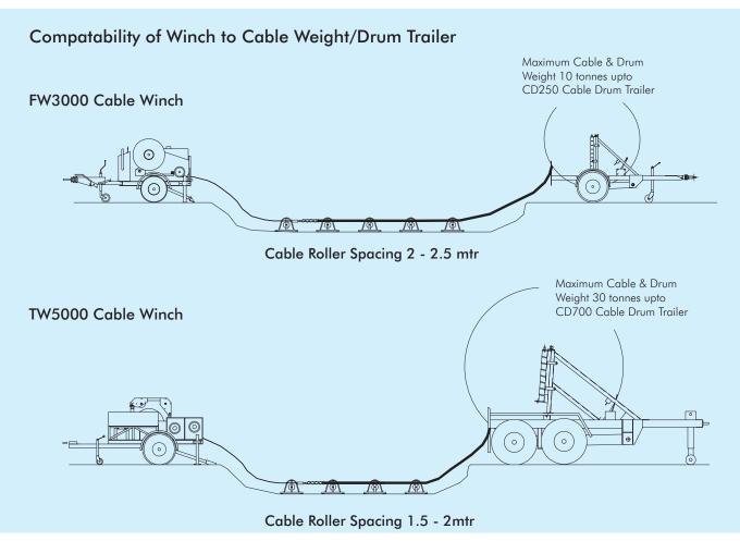
**Important** Do not leave lead sheathed cable on cable rollers over nights as the cable will sag between rollers. This can potentially, cause damage to the cable.
