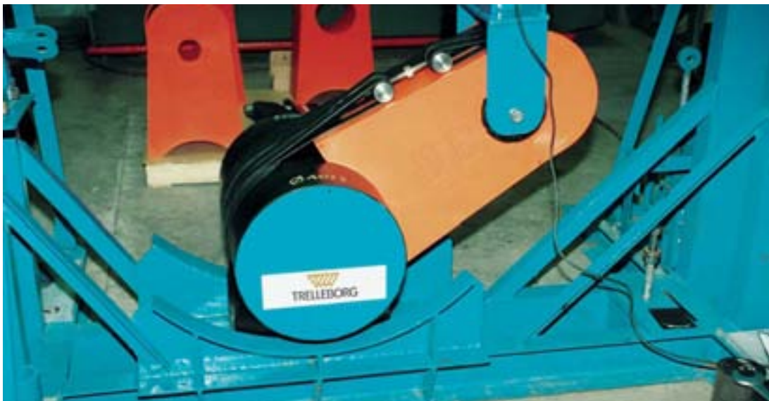
In-house load testing for Factory Acceptance Testing
