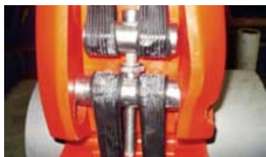
Kevlar Strap and Tensioning Assembly under Load Testing
