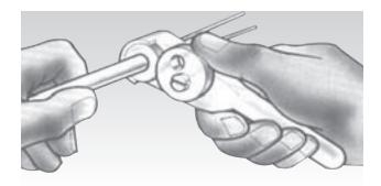
Engage the ratchet wheel into the knurled section of the pot and maintain this contact with thumb or finger as appropriate. Applying forward pressure and a cranking action, screw the pot squarely onto the cable.
