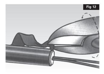
If the insulant has adhered to the conductors this should be removed. The cable is now ready for sealing.
