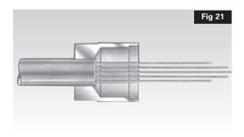
Spread out the outer conductors and push the compound around the inner conductor(s), with thumb behind the paper to ensure cleanliness. At the same time covering the cable face at the base of the pot (Fig. 22).
