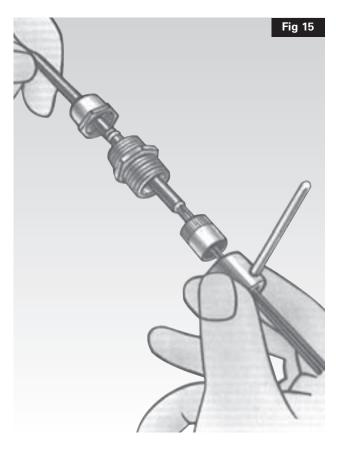
Turn Pyro Potter in a clockwise direction while applying sufficient forward pressure to engage internal screwthread (Fig. 16).
