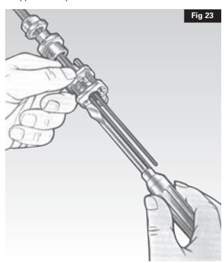
Fully slacken the two screws, slide the crimping plate over the conductors and up to the pot. Swivel the slotted base plate up around the cable behind the pot and tighten the two screws, which will drive the stub cap or disc fully into the pot recess and secure it in position by means of three indent crimps. Slacken the crews and remove the tool (Fig. 23).
