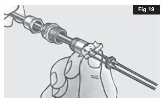
Slide the stub cap or disc/sleeve assembly up to the pot and press it into the pot recess with the aid of a pair of pliers, applying pressure only to the face of the cap or disc (Fig 20).
