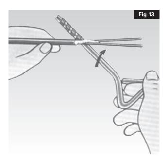
As the insulant has adhered to the conductors this should be removed. The cable is now ready for sealing.
