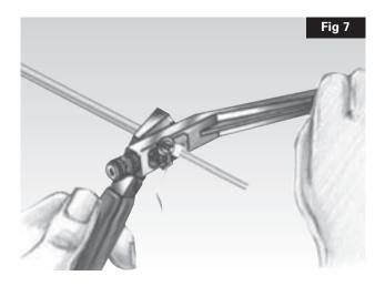
If the insulant has adhered to the conductors this should be removed. The cable is now ready for sealing.
