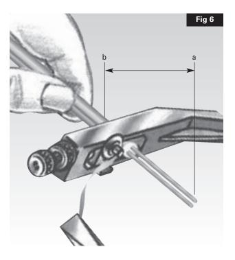
When sufficient sheath has been stripped the operation is terminated by gripping the cable with pliers at the point marked 'b' and allowing the tool to rotate against the jaws (Fig. 7). Remove the tool.
