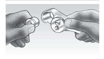
Insert the seal pot open end first into the tool recess.
