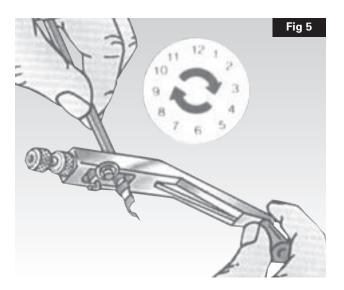
Rotate tool in a clockwise direction applying slight pressure in the direction of stripping until in the case of the ZSU and ZSUS Strippers sufficient swarf has been formed to allow it to be bent round the adjacent post (Fig. 5 and 6). This will prevent the tool snagging the swarf. Once stripping has commenced, all 3 rotary stripping tools will propel themselves along the cable.
