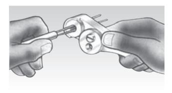
Feed the exposed conductors through the seal pot until the cable sheath is in contact with the self cutting thread of the pot.
