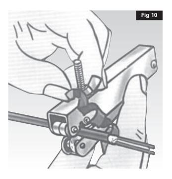
Rotate the cutter around the cable for one complete turn, or more if the first cut appears shallow. The correct depth for the groove is half the thickness of the sheath and reference to Fig. 11 will show the results of over or under cutting.
