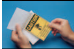
Place marker between the two pieces of self-adhesive laminate liner.
