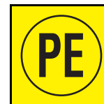
PESC-†-PE Protective Conductor
