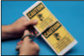
Print paper marker using a laser or ink jet printer and cut out with scissors.
