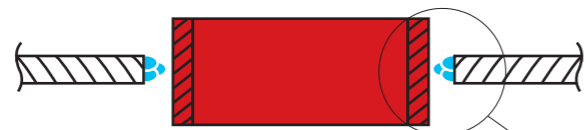
FIG 2: Build-up of fillet joint.
