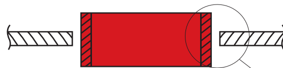
FIG 1: maximum allowable root gap for fillet joint
