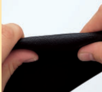
UV Checking: Storing in areas exposed to prolonged sunlight causes UV checking.
