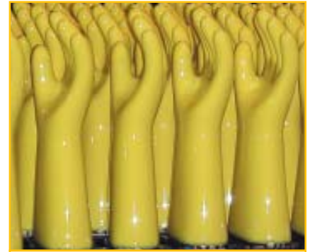
E011Y Gloves being manufactured.
