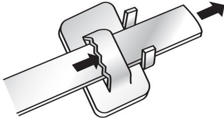
1. Pull appropriate length of band from BAND-IT Tote (approx. 3 1/2 times the diameter of the pole or mastarm for a single-wrapped clamp and seven times the diameter for a double-wrapped clamp. Add 6-8 inches for both single-wrapped and double-wrapped clamps to accommodate the tail and bracket design.) Cut the band using one of the BAND-IT tools with built-in cutter. One end of the band will be very flat and the opposite end will be slightly bent from the cut-off.
