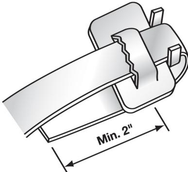
2. Holding the buckle in one hand, with ears pointing upward and to the right as shown, insert the bent or twisted end of the band through the buckle "bridge," past the ears and bend so that at least 2 inches are underneath the buckle.
