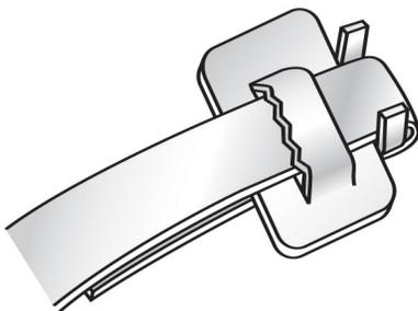
3. Squeeze this "lip wrap" to flatten the bend preventing "pull-out" during tensioning.
