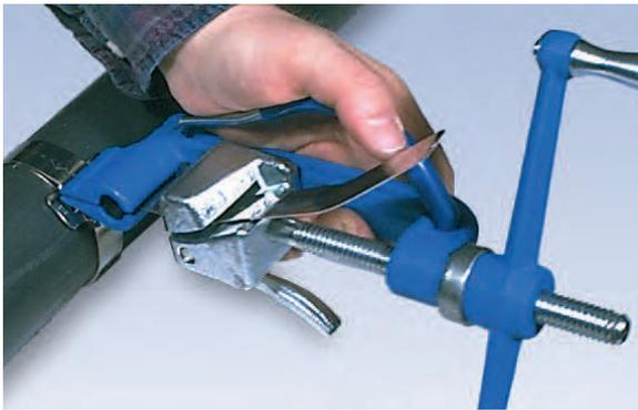
7. To set the lock and cut off band, roll tool nose over buckle, relieving a slight amount of tension by backing off tension handle during this fold over operation. Failure to back off tension handle throughout the entire course of roll over may result in breaking band. On the other hand, releasing too much tension may result in a loose clamp.
