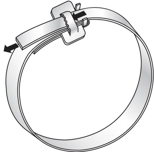
4. Wrap band through sign bracket and around the pole or mastarm and thread through bridge as shown.
