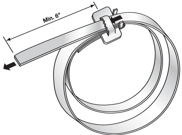
5. Repeat a second wrap of band through the bracket and buckle for a continuous double-wrap application. Double-wrapping develops greater radial compression than single-wrapped clamps and more than doubles the holding strength for heavy objects and high wind loads.
