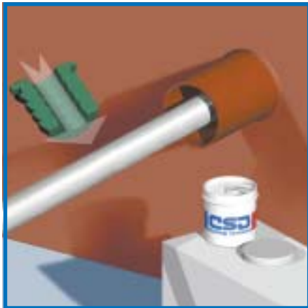
The inside wall of the conduit sleeve and the segments of the sealing plug are treated with CSD® lubricant.
