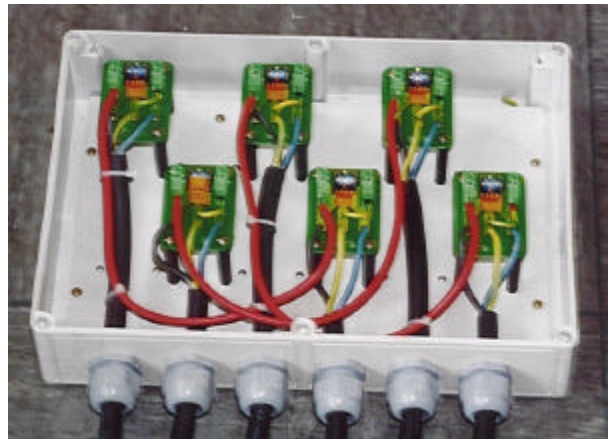
Fig.3: Cross bonding of water sensors
