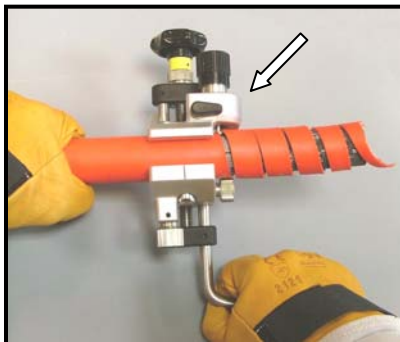
TAKE OUT EXTERNAL SHEATH (when no separator between outer sheath and the aluminum or copper wire, use the stripping plier. Ex: 2028 2152 NI)
