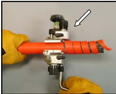
TAKE OUT THE EXTERNAL SHEATH (when no separator between outer sheath and aluminum or copper wire, use the stripping plier. Ex: 2028 2152 NI)
