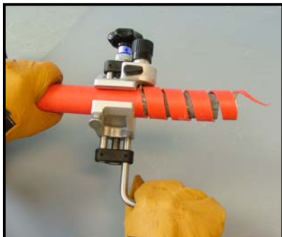
TAKE OUT THE EXTERNAL SHEATH (when no separator between outer sheath and the aluminium or copper wire, use the stripping plier. Ex: 2028 2152 NI)
