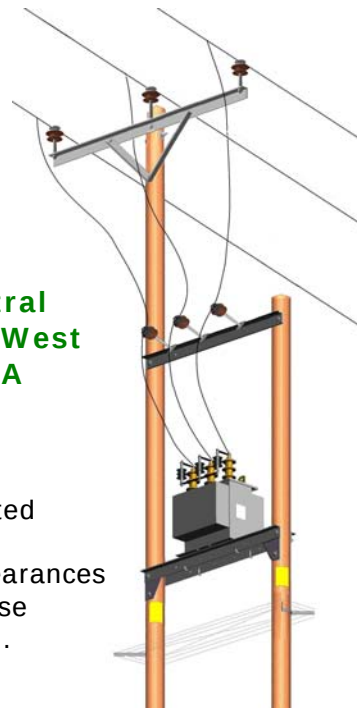
Stub Leg set at a right angle (or at any angle to suit to the situation)
