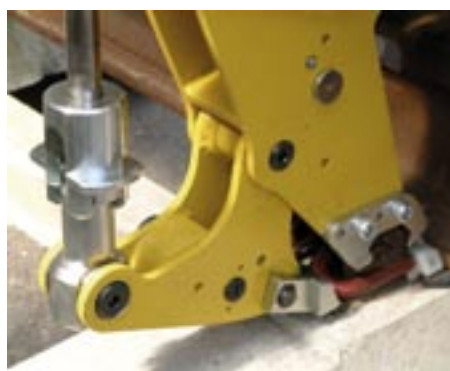
Extraction and insertion of Pandrol "fast clips".
