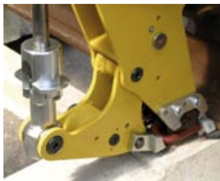
Extraction and insertion of Pandrol "fast clips".
