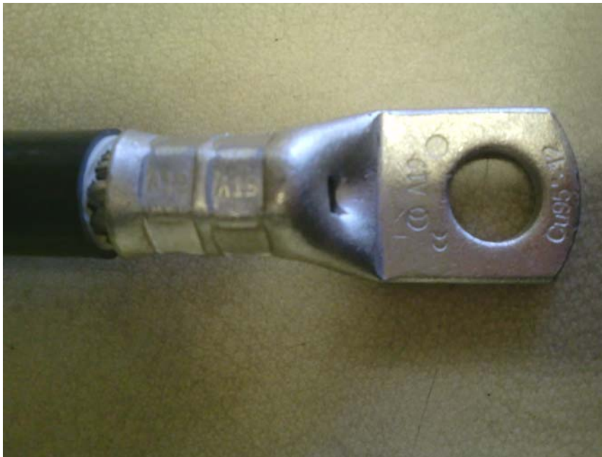
Figure 3. Correctly crimped joint
