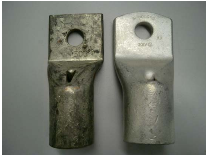
Figure 10. Physical differences between terminal lugs for identical conductor CSA
