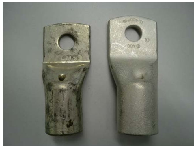
Figure 7. Physical differences between terminal lugs for identical conductor CSA
