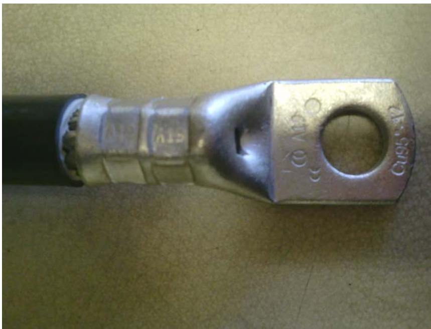
Figure 3. Correctly crimped joint
