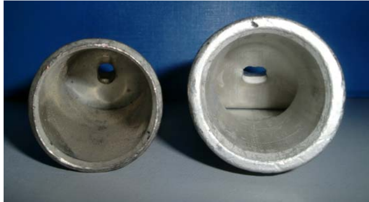
Figure 6. Tube cross section difference. Competitor's terminal lug on left, Cembre lug on right. Competitor's terminal lug cross section contains 38% less copper than Cembre lug.
