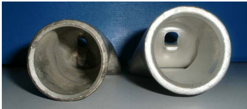
Figure 9. Competitor's terminal lug cross section contains 37% less copper than Cembre lug.
