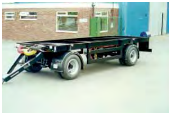
Turntable Steer Trailers - Model shown is 12000Kgs gross fitted with ABS braking to full UK highway specification
