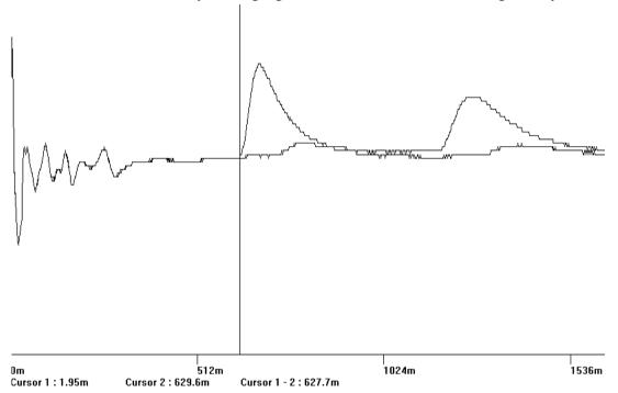
design, or environment (temperature and moisture for example), some cables may show a 'noisy' trace that is difficult to interpret. Comparing a trace on a bad phase to the equally difficult trace on a phase known to be operational will often allow the fault to be detected. TDRs that can show both traces at the same time or even better, mathematically subtracting one trace from the other, make many faults show up very well.
