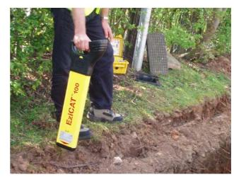
The audio tone changes from pulsed to continuous when electrical current flows
