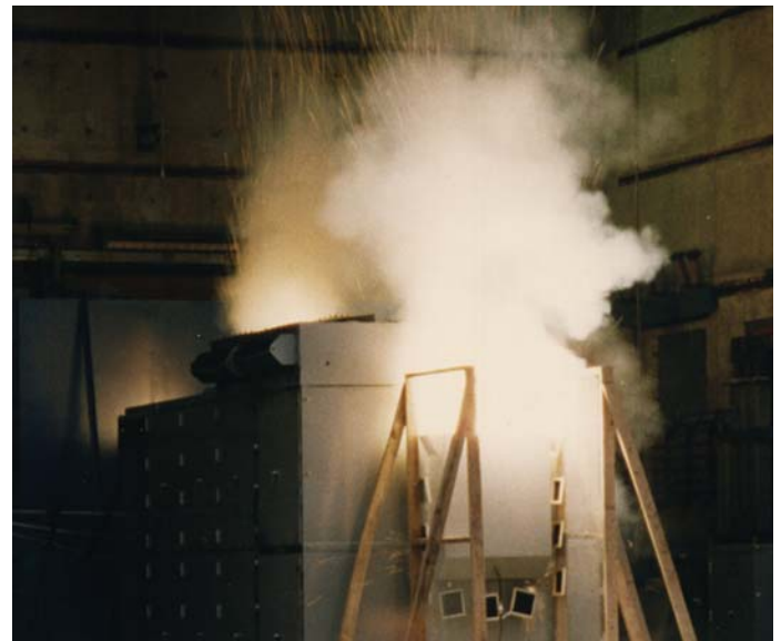
The heat from an arc flash causes the sudden expansion of air
