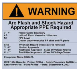
A typical ARC Flash warning label
