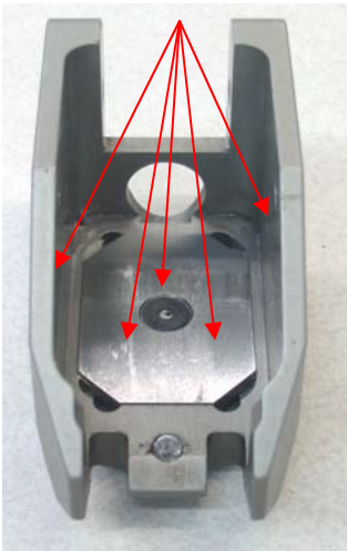
Maintenance Flip Cover every 12,500 cycles
